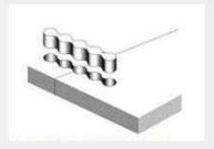
Metalock keys are driven into the opening and caulked.
