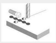
Holes for Metalock screws are drilled along the crack between the keys.
