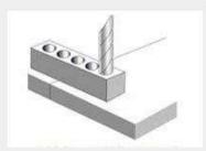
Using a drill jig, rows of blind holes are drilled perpendicular to the direction of the crack, each row to act as a key.
